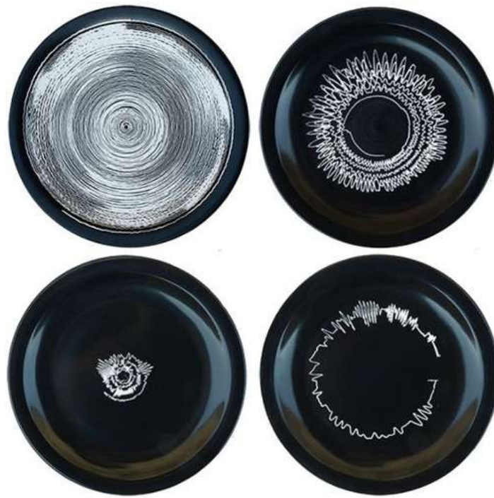
Figure 8.3: Ceramic plate records using custom-built machine for etching sound waves. Source (Segal and Maayan, 2017) .
