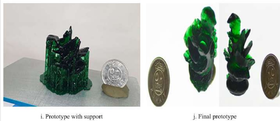
Figure 5.9: Final prototype outputs using UV resin and DLP 3D printer.
