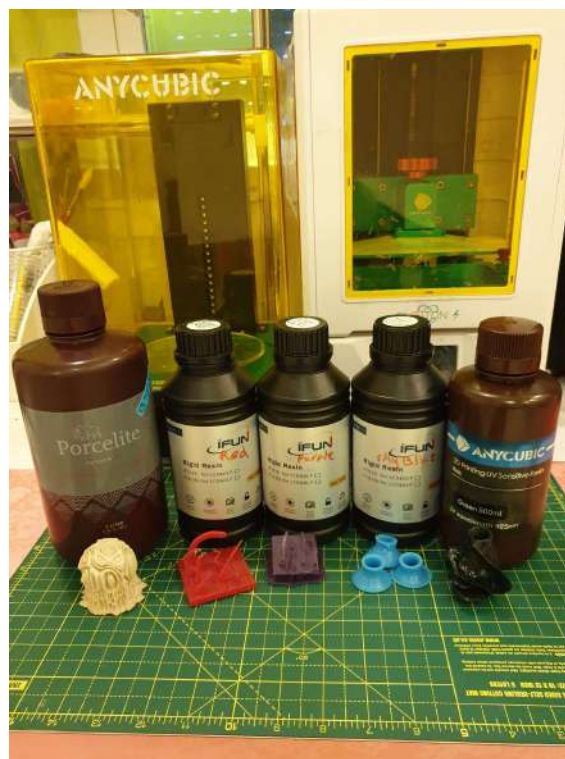
Figure 7.15: UV resin materials used in the experiments of the project
