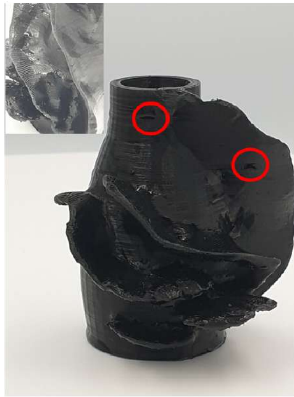
Figure 7.9: Prototype VR model with zero-faces mesh.
