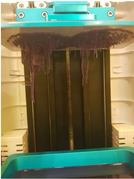
Figure 7.11: Fail support structure test: Slicing 3D model without heavy support and orientation issues.
