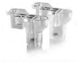
Figure 2.2- MEA Test Cell . Two pairs of electrodes allow a current to be passed across, which when platelets activate and bind, impedance is increased. A Teflon coated stirring bar is used to keep the sample homogenous without increasing platelet activation.
