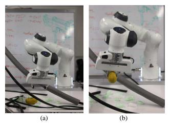
**Fig. 1.** (a) Motion planning and (b) grasping in cluttered environment diffused with rigid and deformable objects.
