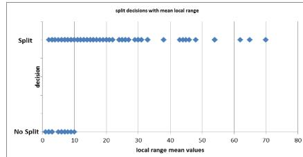
**Fig. 5. Mean values of local range of a  $2N \times 2N$  CU and split decisions.**
