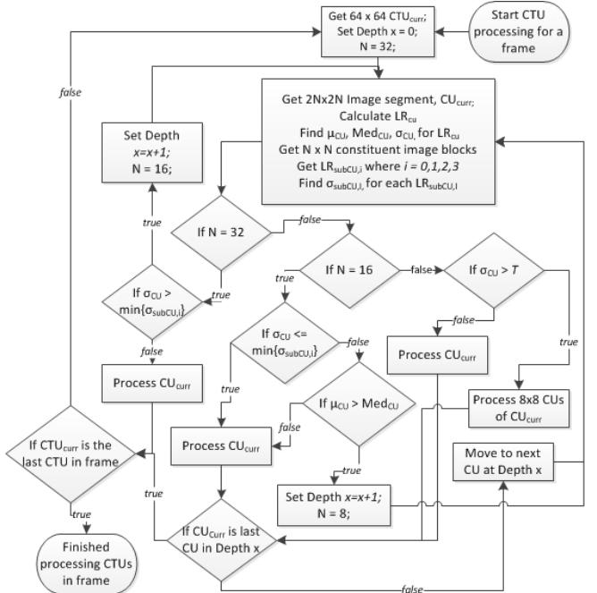
**Fig. 7. CU size determination algorithm using local range and its properties.**
