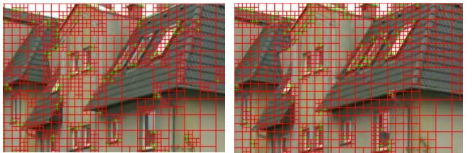
**Fig. 8. Partition structures formed during encoding process. The left figure corresponds to partition structure formed during HM12.0 encoder while the right corresponds to the proposed algorithm.**
