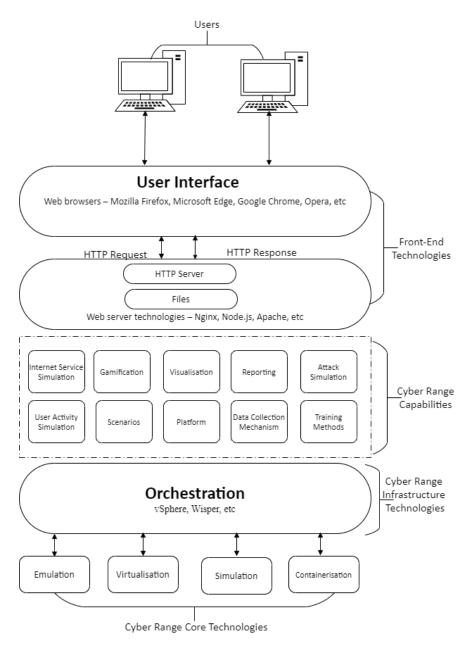
Figure 8. Architectural Design of a Cyber Range.
