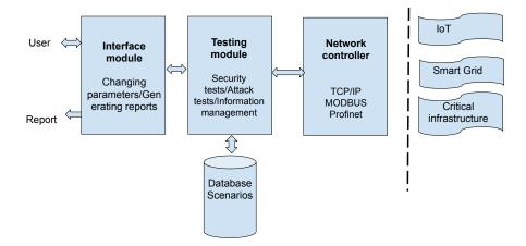
Figure 9. Architectural Design of a Test-Bed.
