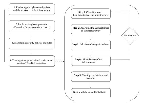
Figure 16. Cyber-range/Test-bed flowchart.
