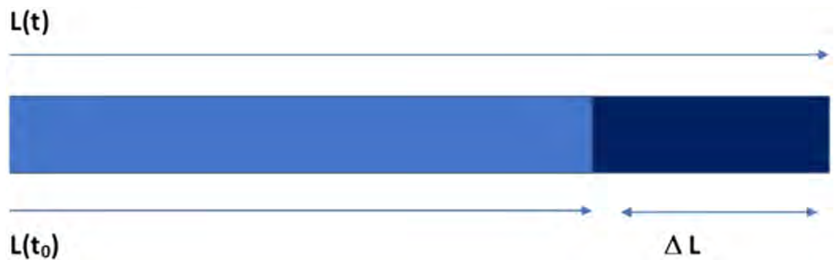
Figure 15. Simple diagram showing the principle of Lagrangian strain.
