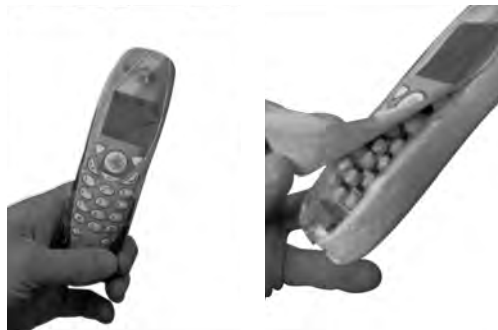
Figure 10 Flat Face low fidelity Equinox model: blue foam with embedded switches covered by a printed sheet of paper
