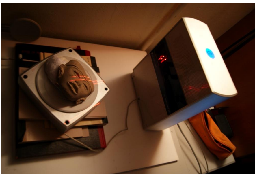
Fig.2 3D scanning of a Mexican artefact at the National Museum Cardiff, using the Next Engine laser scanner; 2013 © Sarah Younan
