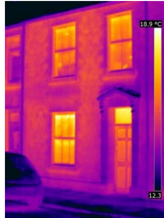
Figure 13: Thermogram of Case study B before installation of EWI
