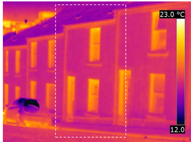
Figure 9: Thermogram of Case study A after installation of EWI
