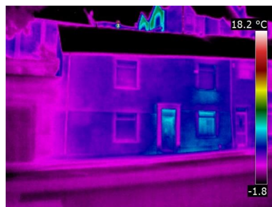
Figure 93: Case Study G Pre-retrofit thermogram
