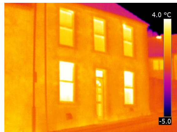
Figure 8: Thermal image of an Arbed case study dwelling before retrofitted EWI was installed
