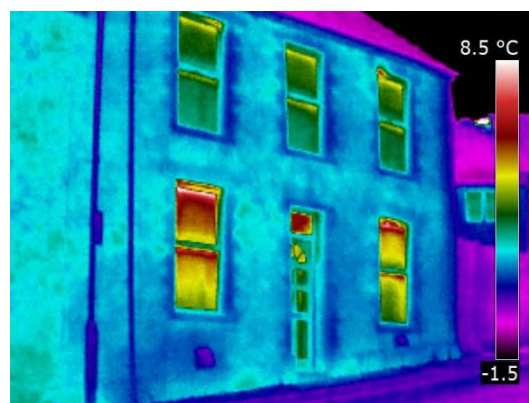
Figure 61: Case Study C Pre-retrofit thermogram
