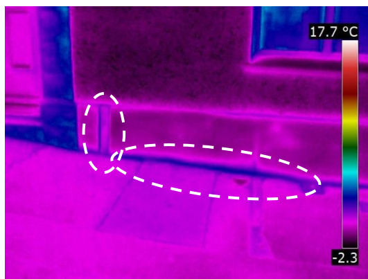
Figure 76: Case Study D thermogram of external wall to pavement junction
