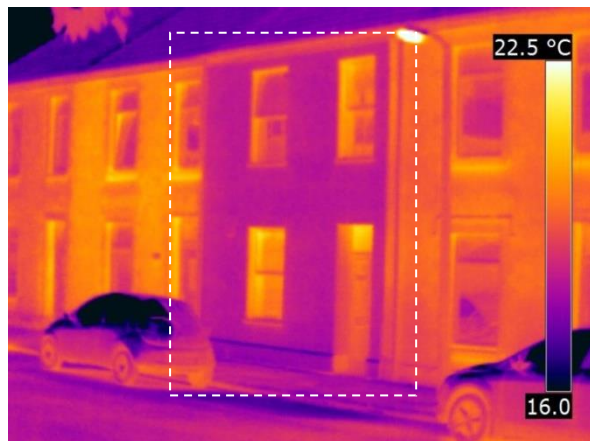
Figure 15: Thermogram of Case study B after installation of EWI
