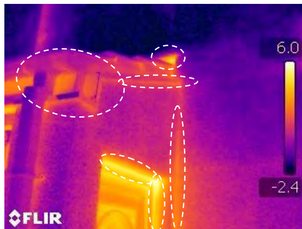
Figure 18: Thermal image showing eaves detail at front porch of case study dwelling (Hopper, 2012)
