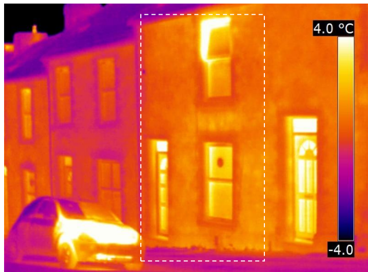
Figure 7: Thermogram of Case study A before installation of EWI
